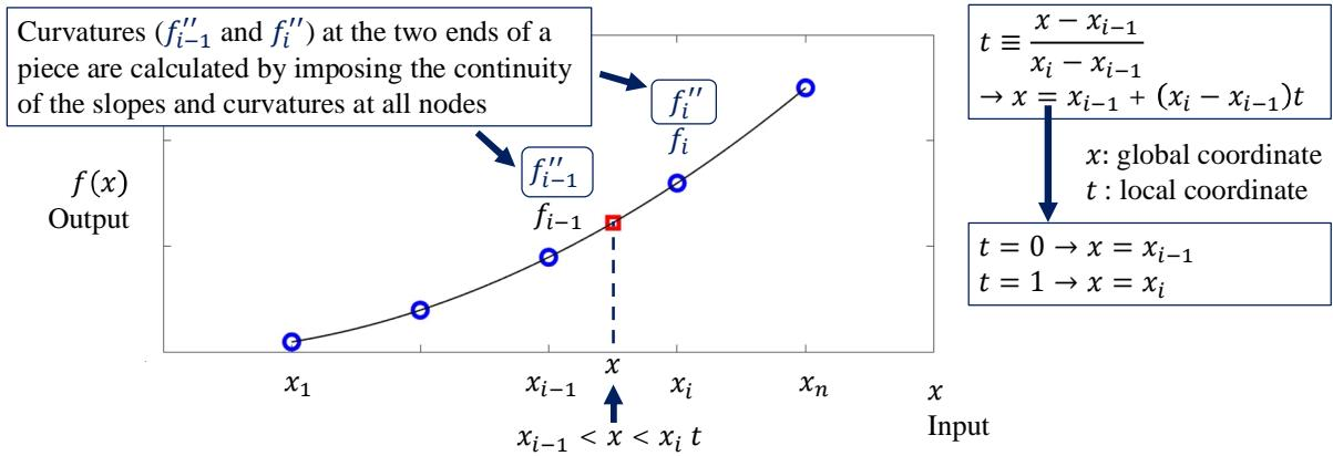
The two unknown curvatures  $f''_{i-1}$  and  $f''_i$  are calculated by solving a system of equations in (Eq.2) for a set of  $n$  nodes.
